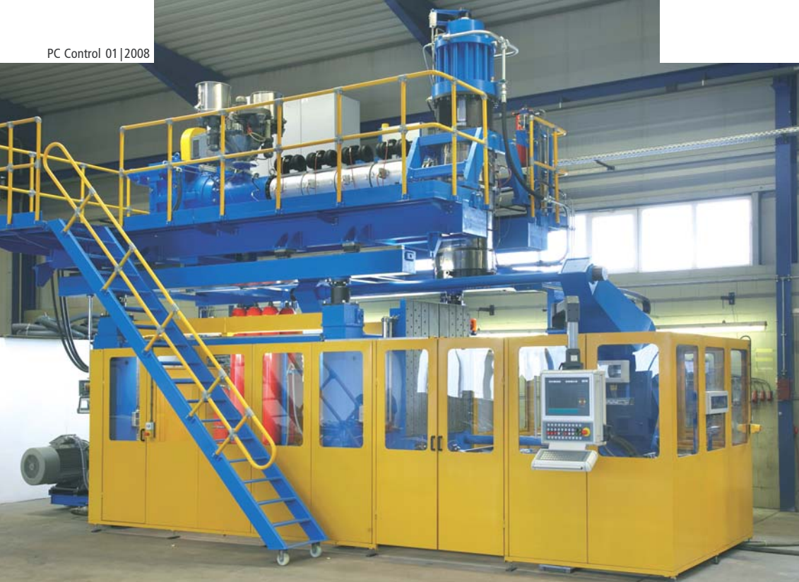
Plastic blow molding machine for producing drums, fuel tanks, and technical components
