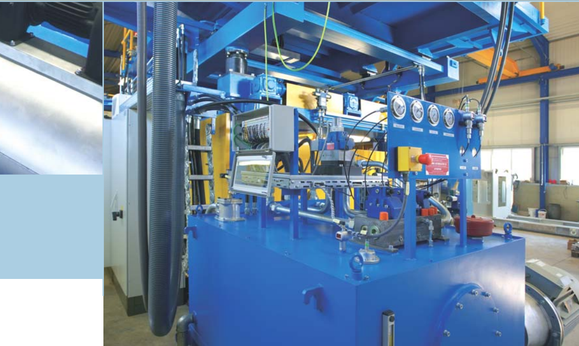
Bus Terminal stations at the extruder, clamping unit, blow station and hydraulic system link the data points locally. The Beckhoff safety terminals offer safety I/O directly in the Bus Terminal station of the system.
