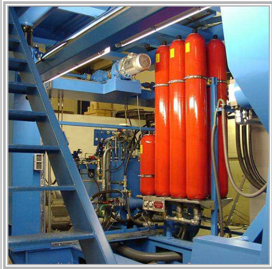
B-750: hydraulic with accumulators
