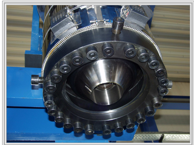
B-750: view into 20 liter accu head
