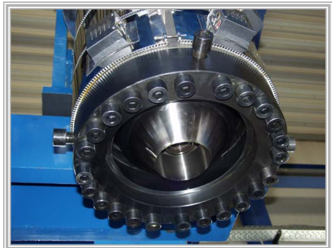
B-750: view into 20 liter accu head
