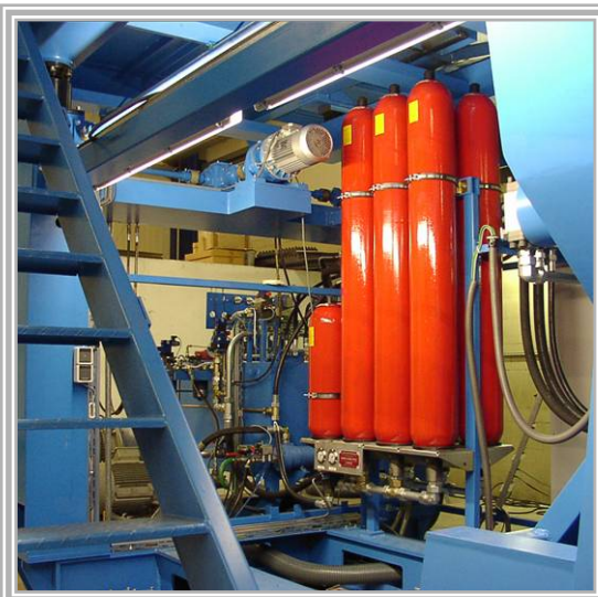
B-750: hydraulic with accumulators
